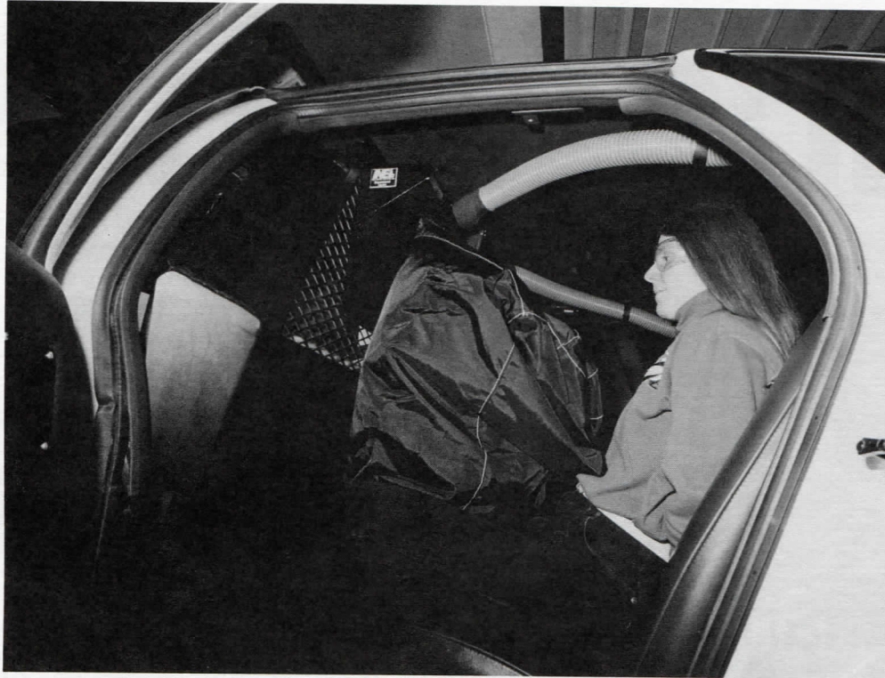
A backseat airbag for police cars to help restrain out-of-control suspects is one of the new technologies developed in federal laboratories. The device is made from a special fiber that allows the person to breathe but restricts movement.
